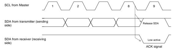
After transmitting the ACK signal, if the Master remains the receiver for transfer of the next byte, the SDA is released at the falling edge of the clock corresponding to the 9th bit of data on the SCL line. Data transfer resumes when the Master becomes the transmitter.
